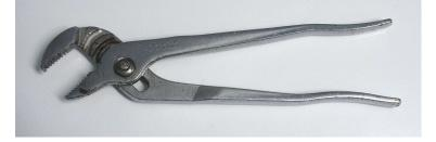
If you don't happen to have these then just use any pliers with jaws wide enough to fit over the metal fitting on the end of the hose.
